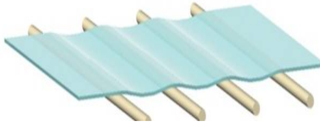
Figure 2. Waviness during glass heating.
