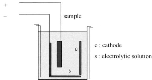
Imagen 1. Schematic representation of the electrolysis process
