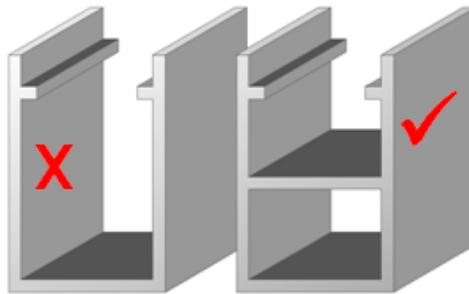
The reinforcement can control the tolerances and gives greater strength to the profile.
